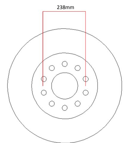
disc is directly mounted on wheel hub
