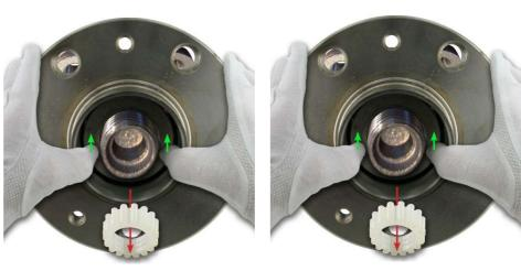
Bearing with plastic Joining sleeve
