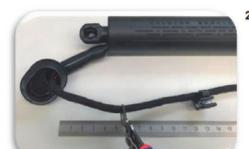
Cut the wiring harness of the original drive about 5cm (2 inches) behind the grommet.
