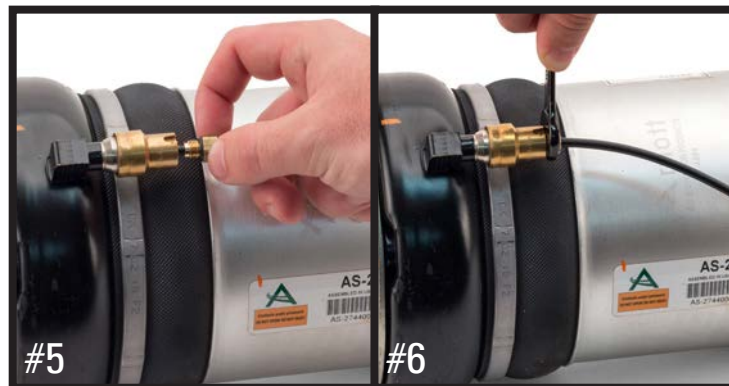
#5 INSERT FITTING AND AIRLINE INTO AIR SPRING
