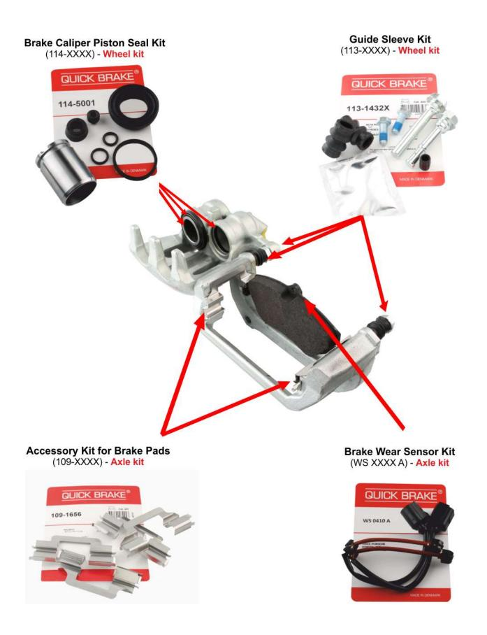
When repairing the Caliper, for technical and safety reasons, it is recommended also to change the Brake Caliper Piston Seal Kit, the Guide Sleeve Kit, the Accessory Kit for the Brake Pads and the Wear Sensor Kit. This to ensure even braking ability and functionality.
